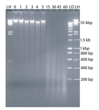
FIG. 6—HL60 DNase degradation series (EtBr-stained). Lanes labeled 0 to 60 indicate DNase treatment time in minutes. Lanes labeled LH and LD represent  $\lambda$ -HindIII and low-mass DNA ladder, respectively.
