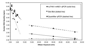
FIG. 7—Nuclear quantifications of DNase-degraded HL60 samples by nuTH01-mtND1 duplex qPCR, Quantifiler<sup>TM</sup> qPCR, and slot blot hybridization. For the qPCR assays, each point represents the average of duplicate quantifications. For slot blot, each point represents a single quantification. Lines represent linear least-squares fits to early (0–5 min) and late (15–45 min) time points in the degradation series.
