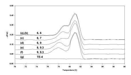
FIG. 4—SYBR<sup>®</sup> Green melting curves obtained for DNA extracts from six different individuals and a negative control sample using the TH01 qPCR assay. The TH01 genotype for each sample is indicated. Traces (a) and (b) are from two different individuals, both genotype 6, 6 at TH01.
